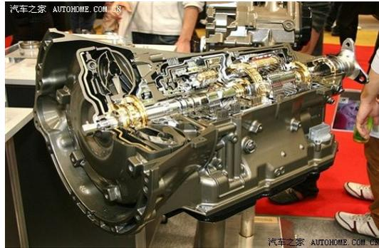
The AA80E is Aisins High Torque Automatic 8 Speed transmission, and is currently used by several manufacturers today. This Document deals with the version fitted to the Lexus IS-F models.
